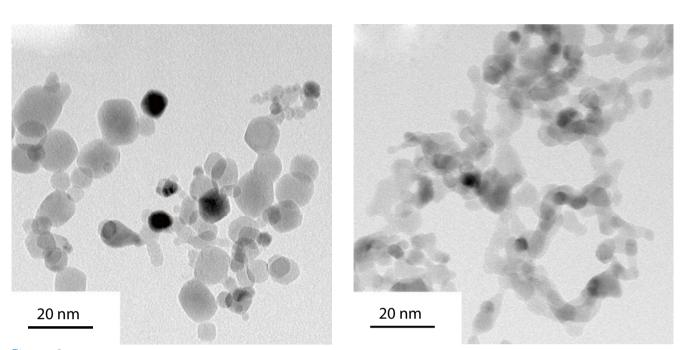
Figure 3 Transmission electron microscope images of ZrO<sub>2</sub> from a flame spray pyrolysis unit (left) and a pulsation reactor (right) (© IBU-tec)
