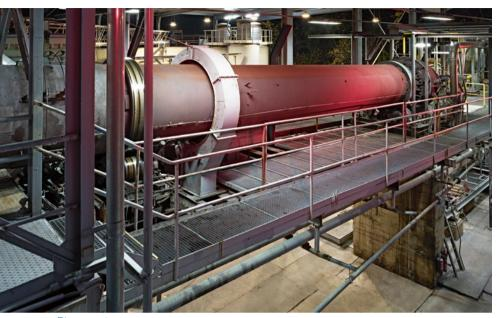
Figure 4 The directly fired rotary kiln (GDO) at IBU-tec (© IBU-tec)
